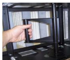
Gasketed doors and easy service HEPA clamp
