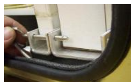
Gasketed doors and easy service HEPA clamp
